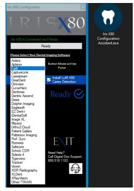
Launch Video in Cadi, in the Device Setup Window, go to Expert Settings and Modify the preferences to match the table below.
