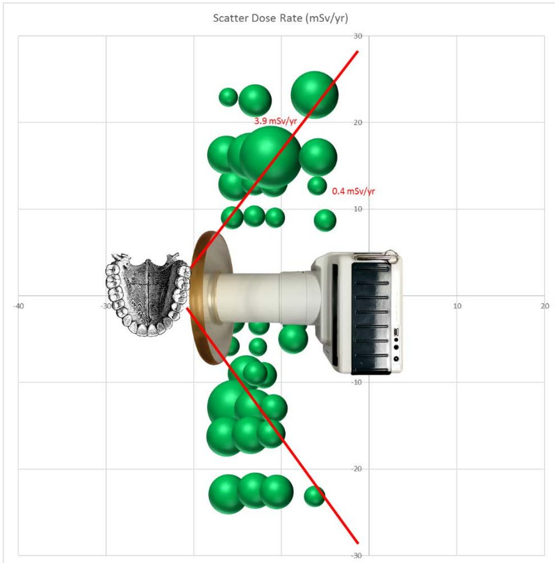
**Figure 7b. Side view with dose rates of 3.9 and 0.4 mSv/yr labeled for comparison. Bubbles indicate the magnitude of dose rate relative to their surface area.**
