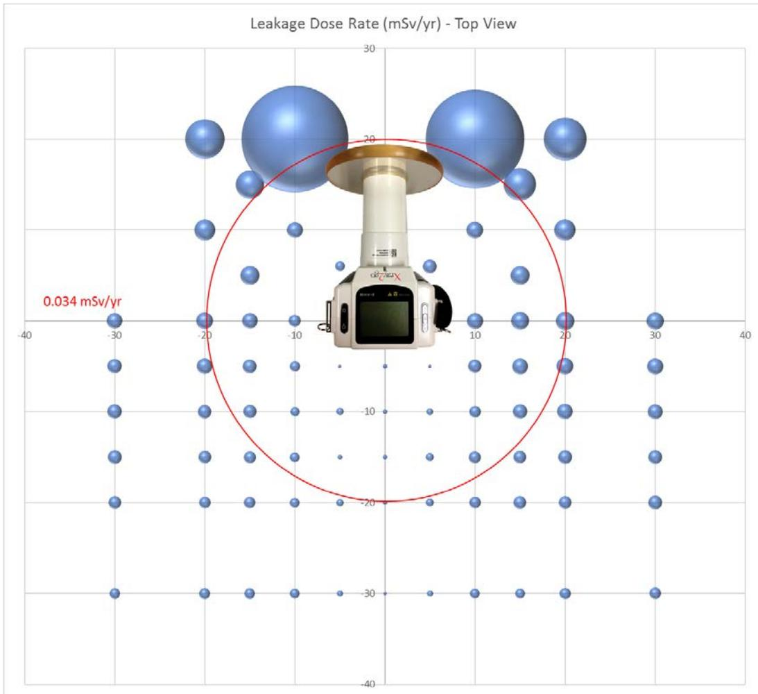
**Figure 4b. Top view. Bubbles indicate the magnitude of exposure relative to their area. The red circle simply indicates a distance of 20 cm from the focal spot, and the value provided in red gives the reader an indication of relative dose rates for all other measurements.**
