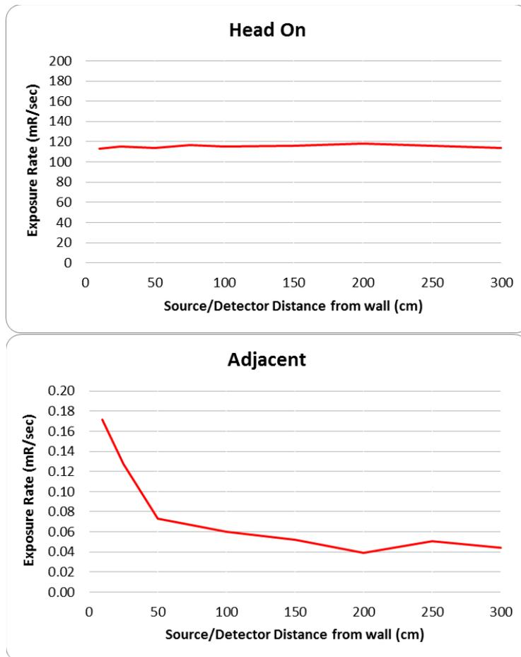
**Figure 1. Influence of scatter from (a) head on and (b) adjacent measurements of exposure.**
