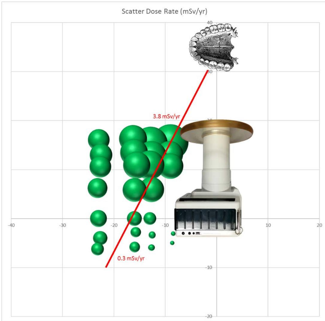
**Figure 8. Side view with dose rates of 3.8 and 0.3 mSv/yr labeled for comparison. Bubbles indicate the magnitude of dose rate relative to their surface area. There is now a 10 cm gap between the end of the collimating tube and the patient's cheek.**
