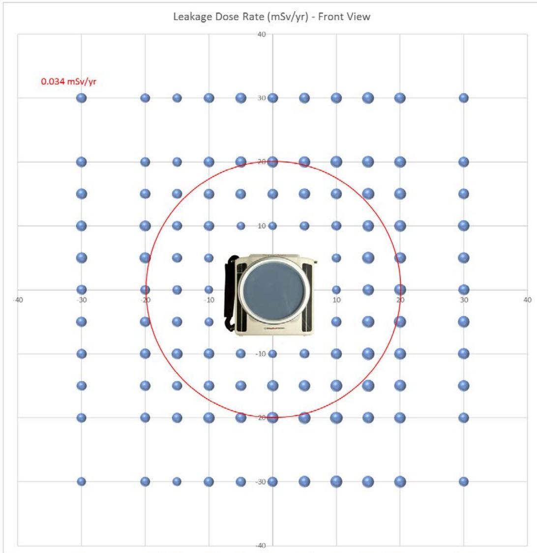
**Figure 4a. Front view where the primary beam of X-rays is coming out of the page. Bubbles indicate the magnitude of exposure relative to their area. The red circle simply indicates a distance of 20 cm from the focal spot, and the value provided in red gives the reader an indication of relative dose rates for all other measurements.**
