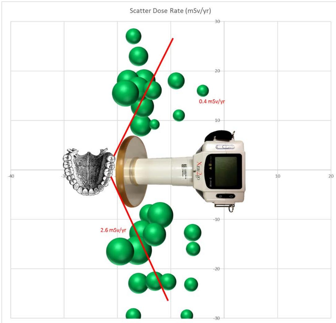
Figure 7a. Top view with dose rates of 2.6 and 0.4 mSv/yr labeled for comparison. Bubbles indicate the magnitude of dose rate relative to their surface area.
