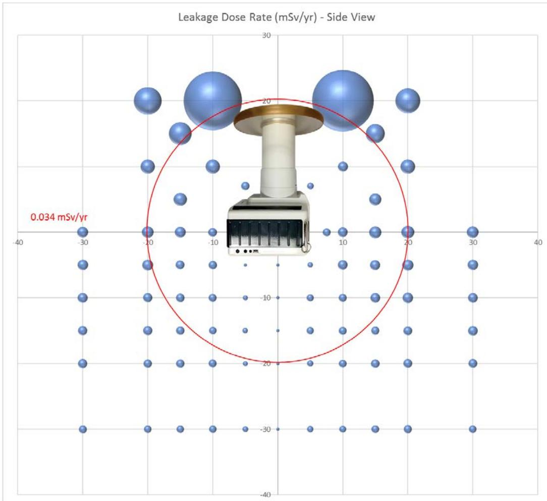
**Figure 4c. Side view. Bubbles indicate the magnitude of exposure relative to their area. The red circle simply indicates a distance of 20 cm from the focal spot, and the value provided in red gives the reader an indication of relative dose rates for all other measurements.**
