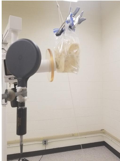
**Figure 6. Orientation of the Xray2Go, the alpaca skull, and the ion chamber during backscatter measurements.**
