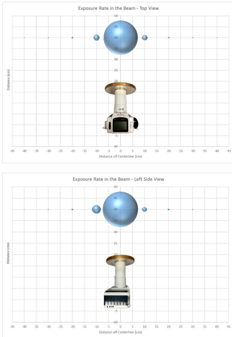
**Figure 9. (a) Top view and (b) side view. Beam exposure rate at a distance of 40 cm from the focal spot is 62 mR/sec. Bubbles indicate the magnitude of exposure relative to their surface area.**
