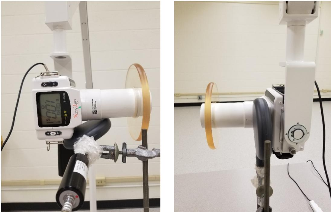
**Figure 3. Demonstration of contact leakage-exposure measurement.**
