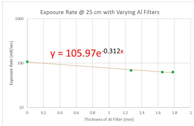
**Figure 11. Exposure rate in the beam for 60 kV @ 2 mAs from the Xray2Go (MiniX-S) as a function of aluminum thickness placed into the beam. Distance from focal spot to detector is constant.**
