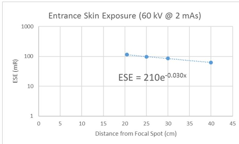
**Figure 10. Entrance Skin Exposure (ESE) for 60 kV @ 2 mAs from the Xray2Go (MiniX-S) as a function of distance from the focal spot.**
